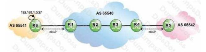
AS 65540 is using MPLS to provide BGP shortcuts for its iBGP routing. Which routers must be configured with the "configure router bgp igp-shortcuts rsvp-te" command?
