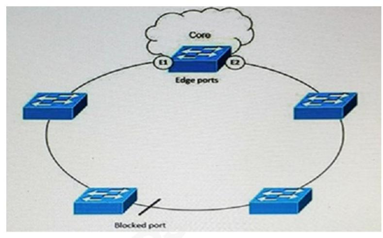
Refer to the exhibit. As the new network designer for a manufacturing company, you are designing this resilient Ethernet ring for the plant Ethernet network that is connected to the core, which does not use STP. Both edge ports are on the same switch in a ring segment. There is connectivity between the edge ports throughout the segment, so you create a redundant connection between any two switches in the ring. Which four options are characteristics of this design? (Choose four.)
