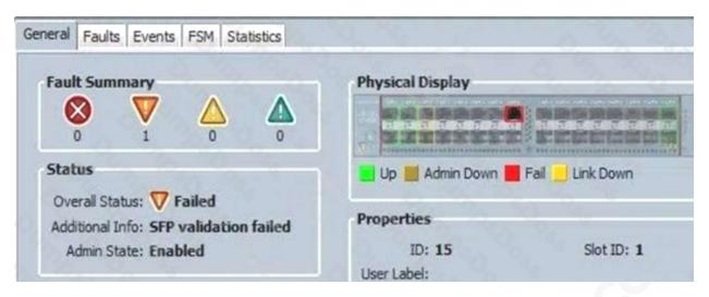
Refer to the exhibit. When an engineer inserts 8-Gb Fibre Channel SFP port 15 on a Cisco UCS Fabric Interconnect, the port fails. What is causing this issue?
